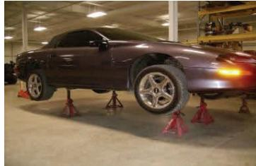
1. The vehicle must be supported by the chassis structure as close to the suspension mounting points as possible. Support the vehicle near the forward lower control arm pockets in the rear and the suspension mounting points in the front. This must be done on a hard level surface.
