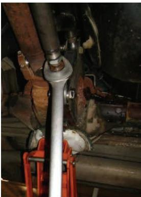
15. At this time the pinion angle needs to be set. To do this the weight of the vehicle needs to be on the rear suspension. This can be accomplished by moving the rear jack stands under the rear axle housing. Keep the vehicle as level as possible during this procedure.
