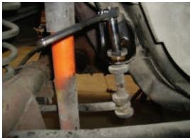
3. Remove the sway bar end links. A little bit of penetrating oil on the threads during disassembly will help.
