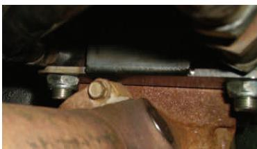
12. using the supplied hardware, attach the torque arm adapter to the rear axle assembly. Make sure you allow adequate clearance from the pinion yoke to the torque arm adapter bracket. **Note;** when attaching the torque arm adapter to a Moser Engineering 12 bolt axle assembly it is imperative that you use a thread locker on the attaching hardware. Proper preparation of the housing and associated hardware is an absolute necessity to insure
