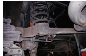
5. Lower the rear axle assembly just enough to remove the rear coil springs from their pockets. Make sure not to damage the rear brake hose or hoses during this process. On some applications it may be necessary to disconnect the rear brake hose from the vehicle. Be very careful during the removal of the rear springs, they're under an extreme amount of compression! Once the rear axle assembly has been lowered enough to remove the springs, slide them from their pockets.
