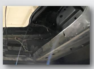
To install the subframe, you'll need to remove the spring pockets and supporting gussets and anything else that might obstruct the installation of the subframe. This can be accomplished by using a spot weld drill. They can be purchased at most auto supply stores. In our prototype vehicle we removed the floors from the pinch weld on the crossmember just in front of the differential to the tail light panel. We did this for ease of design, it's not necessary to complete this project.
