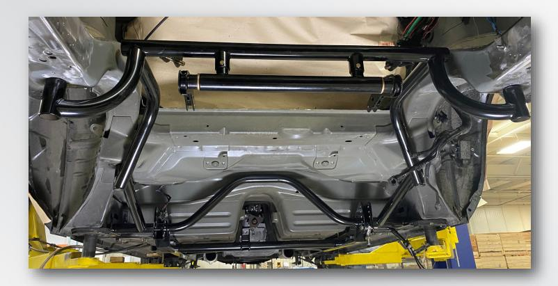
Make sure the weld plates on the end of the crossmember are clean as well. Once everything is clean, re install the sub frame. In preparation for welding, it may be necessary to use a jack to push the crossmember weld plate tight against the bottom of the rocker. Be extremely careful doing this, you don't want to knock the car off of the supports! Tack each side in place before completing any welding.
