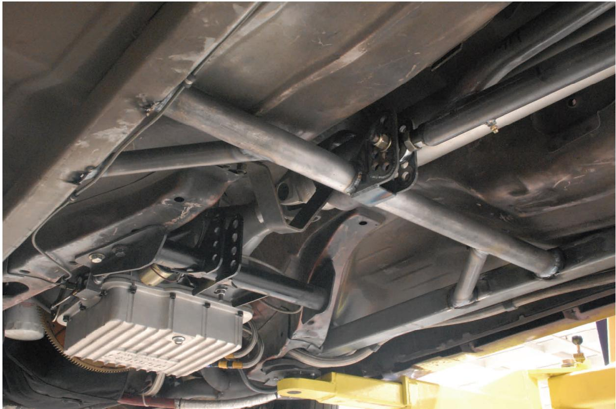
The center section and driveshaft need to be temporarily installed to determine that there is at least  $\frac{1}{4}$ " of clearance from the torque arm and driveshaft. Also make sure the torque arm to the jam nut on the slider is still at 1". With all of these conditions met, install the 1 1/4:" diagonal from the chassis to the crossmember. Finish weld all attaching points.
