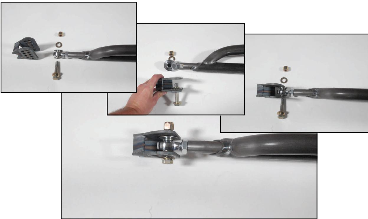
With the mount properly positioned, measure the location of the 1 3/4" cope at the front of the mount in reference to the vehicle so the cross member can be properly located.
