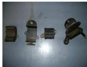
8. The factory rubber bushings need to be removed from the clamshell mount. A new poly bushing will take their place during the installation process. Center punch the rivet heads and drill through the rivets to remove the rubber from the clamshells.
