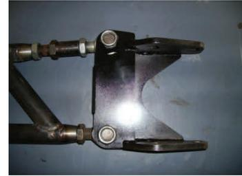
11. Attach the torque arm adapter to the rod ends using the supplied 3/4" hardware. The nylon lock nuts need to be on the driveshaft side of the bracket to prevent them from rubbing on the driveshaft tunnel.
