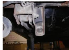
4. Remove the lower rear shock mount nuts.
