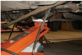
2. The rear springs must be removed the vehicle to keep the housing from rotating during the installation of the replacement torque arm. Support the rear axle assembly during the installation process.
