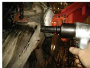
7. Remove the two thru-bolts that attach the rear part of the torque arm to the axle housing. Remove the torque arm from the vehicle.
