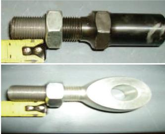
9. Start with the installation of the jam nuts on the pinion angle adjuster and the solid rod ends. The jam nuts thread on to 7/8". The jam nut on the adjuster is LH thread, the jam nuts on the solid rod ends as RH thread.
