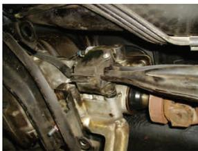
6. The forward torque arm mount is a 2 piece clamshell design with rubber inserts riveted to the clamshell mount. The outer half of the clamshell mount must be removed to remove the torque arm from the vehicle.
