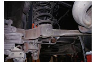
5. Lower the rear axle assembly just enough to remove the rear coil springs from their pockets. Make sure not to damage the rear brake hose or hoses during this process. On some applications it may be necessary to disconnect the rear brake hose from the vehicle. Be very careful during the removal of the rear springs, they're under an extreme amount of compression! Once the rear axle assembly has been lowered enough to remove the springs, slide them from their pockets.
