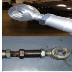
10. Start with the installation of the pinion angle adjuster into the lower tube adapter. Use an anti seize lubricant or heavy grease to prevent the threads from galling during this process. Thread the adjuster in the adapter until the jam nut just touches the adapter. Repeat this process with the solid rod ends. Do not tighten the jam nuts at this time, this will be done when the pinion angle is set.
