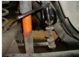
3. Remove the sway bar end links. A little bit of penetrating oil on the threads during disassembly will help.
