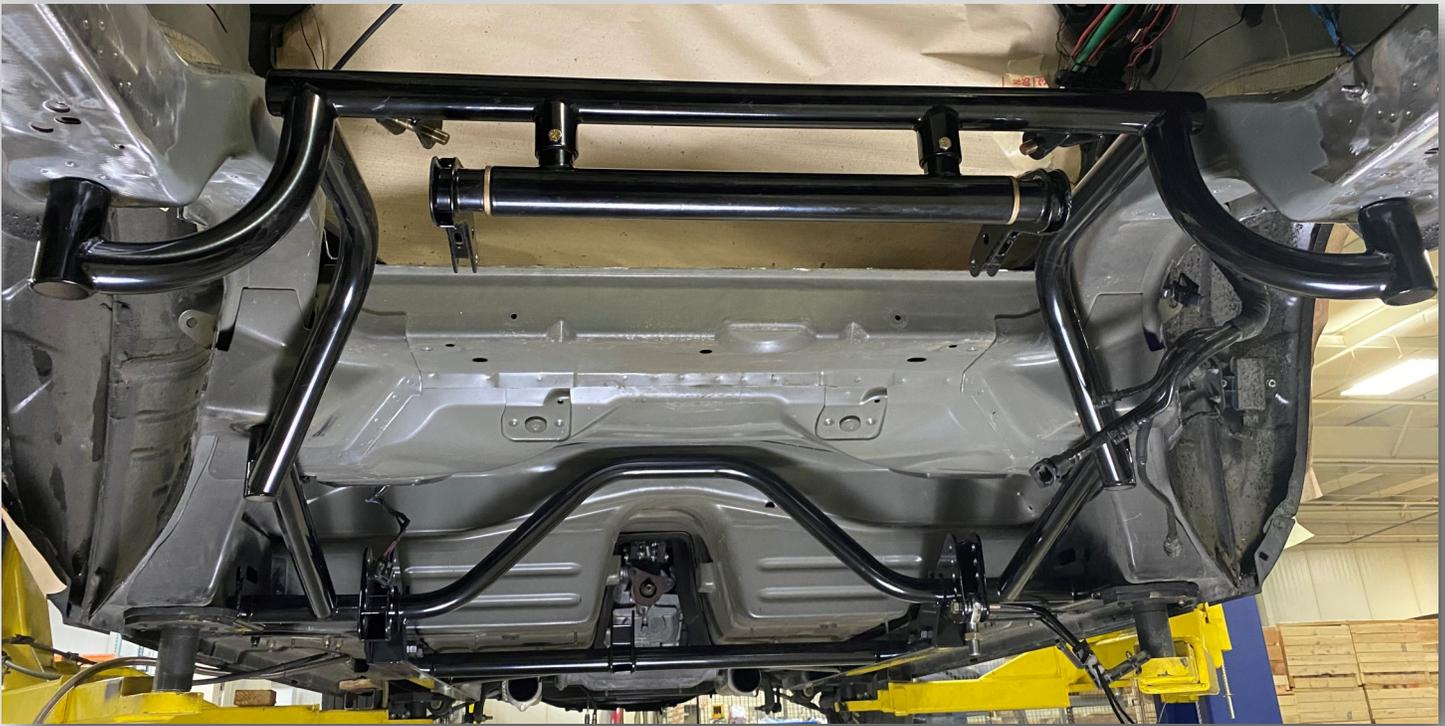
Make sure the weld plates on the end of the crossmember are clean as well. Once everything is clean, re install the sub frame. In preparation for welding, it may be necessary to use a jack to push the crossmember weld plate tight against the bottom of the rocker. Be extremely careful doing this, you don't want to knock the car off of the supports! Tack each side in place before completing any welding.
