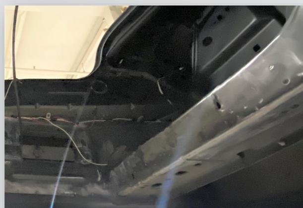
To install the subframe, you'll need to remove the spring pockets and supporting gussets and anything else that might obstruct the installation of the subframe. This can be accomplished by using a spot weld drill. They can be purchased at most auto supply stores. In our prototype vehicle we removed the floors from the pinch weld on the crossmember just in front of the differential to the tail light panel. We did this for ease of design, it's not necessary to complete this project.
