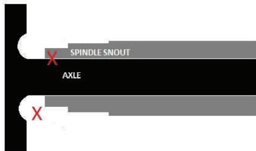
Moser Engineering Alloy floater axles are **NOT** tapered like the stock axles. Be sure to check for clearance at the "**X**" points!
